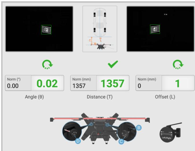
**Figure 6-7 Adjust the Calibration Frame**
