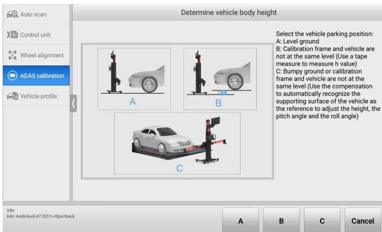
**Figure 6-74 Select Vehicle Parking Position**
