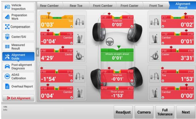
**Figure 4-57 Alignment Result Screen**
