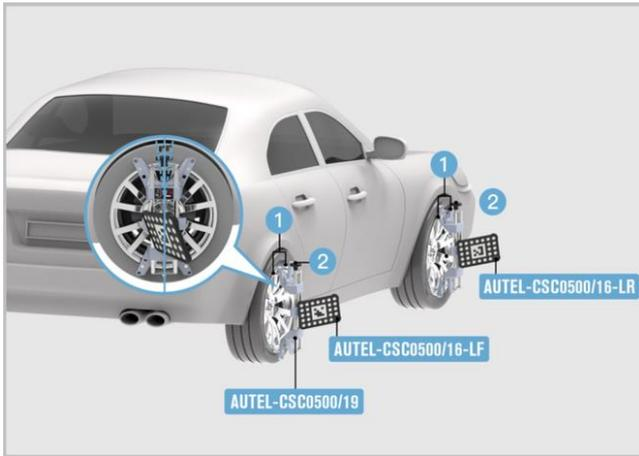
**Figure 6-39 Install Wheel Clamps (Rim Clamps)**
