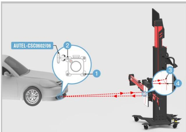
**Figure 6-17 Align Reflected Laser with Origin Laser**
