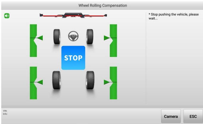
**Figure 5-49 Wheel Rolling Compensation 4**
