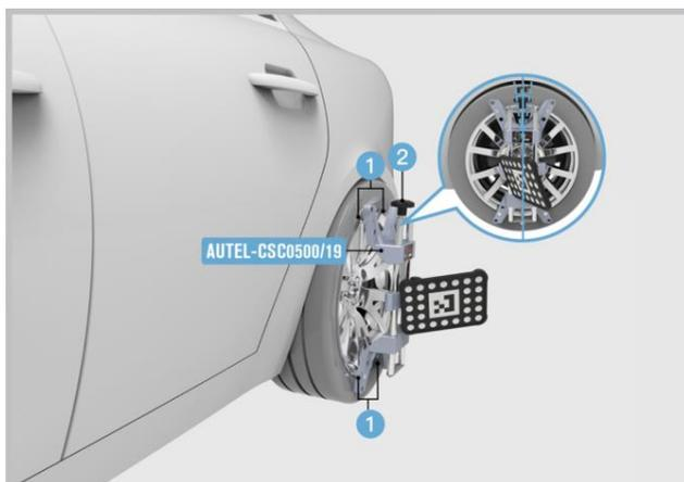
**Figure 6-5 Install the Wheel Clamps (Rim Clamps)**
