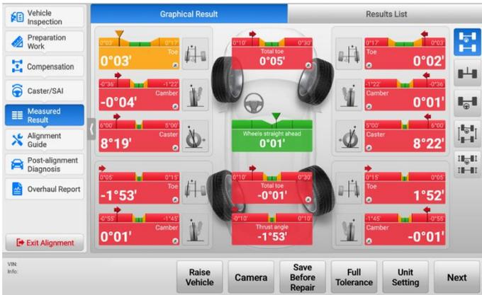
**Figure 4-48 Measured Result Screen (Graphical Result)**
