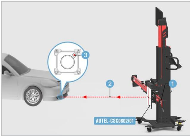
**Figure 6-16 Align Laser with Mini Reflector**
