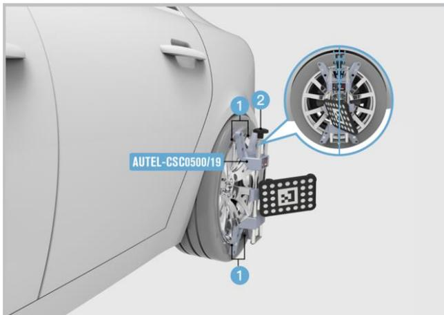
**Figure 6-67 Install the Wheel Clamps (Rim Clamps)**
