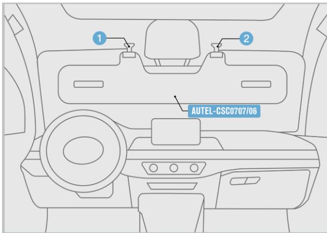
**Figure 6-60 Place HUD Calibration Board**
