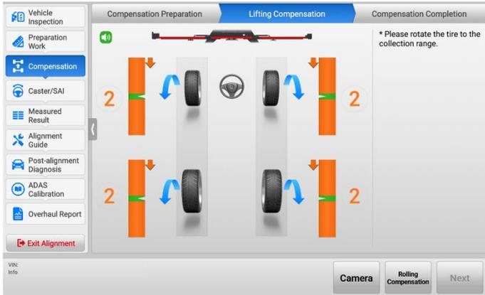
**Figure 4-44 Start Lifting Compensation 3 (Use Rim Clamp)**
