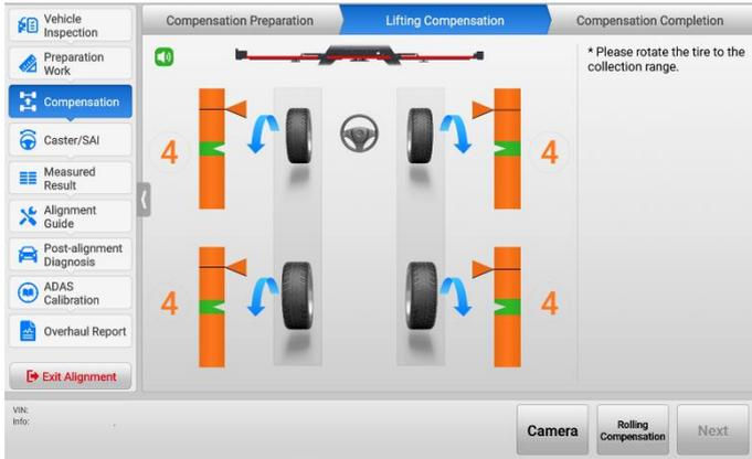
**Figure 4-42 Start Lifting Compensation 1 (Use Rim Clamp)**
