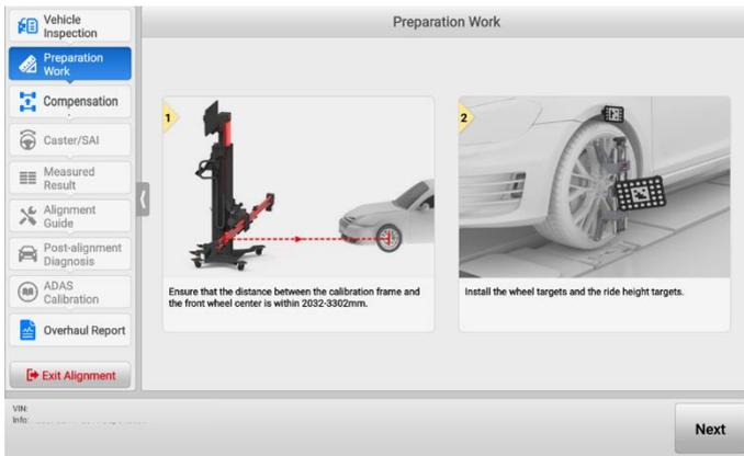
**Figure 4-32 Install Ride Height Target**
