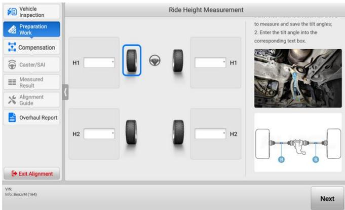
**Figure 4-34 Measure and Input Tilt Angles**
