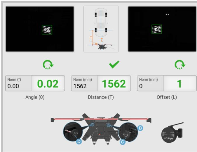
**Figure 6-97 Position the Calibration Frame**
