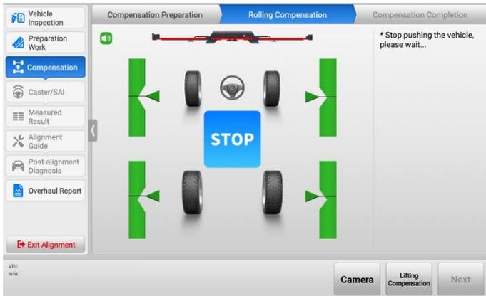
**Figure 4-39 Start Rolling Compensation 4 (Use Rim Clamp)**
