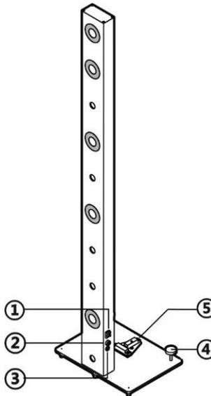
**Figure 3-22 NV Calibrator (Benz) AUTEL-CSC0803/01**
