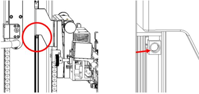
Maintenance method: locate the 2 oil filling ports (as the picture shows) from the gaps on both sides of the calibration frame and use a grease gun to fill them.
