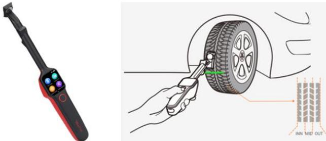
**Figure 4-18 MaxiTPMS TBE Device (not included) and Use Diagram**
