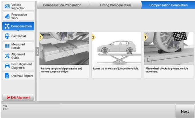
**Figure 4-46 Complete Lifting Compensation (Use Rim Clamp)**
