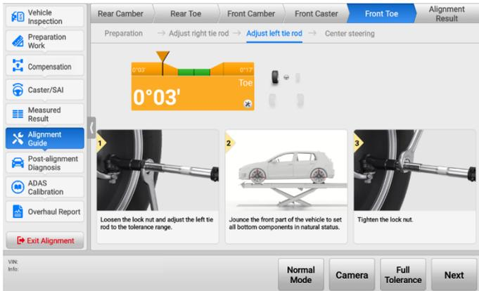
**Figure 4-60 Adjust Left Tie Rod**
