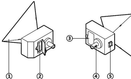
**Figure 3-18 Corner Reflector AUTEL-CSC0802/01**
