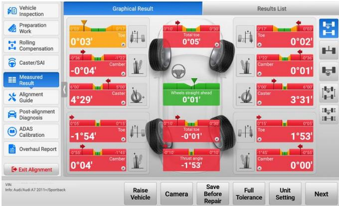
**Figure 5-65 Measured Result (Half Tolerance) Screen**
