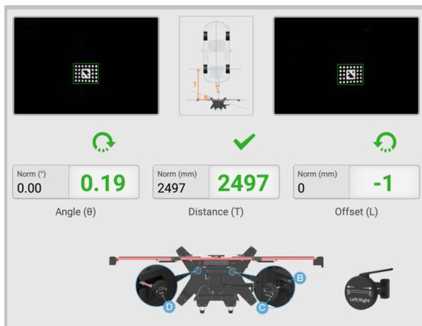
**Figure 6-44 Position the Calibration Frame**
