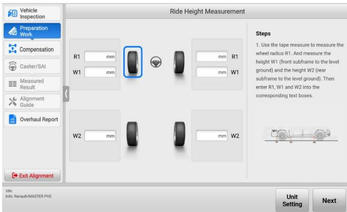
**Figure 4-31 Measure Ride Height with Tape 2**
