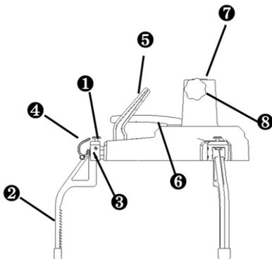
**Figure 3-7 Wheel Clamp (Tire Clamp) AUTEK-CSC0500/17**
