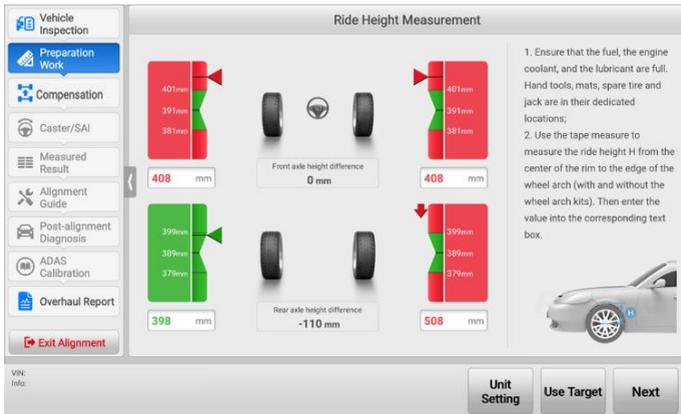
**Figure 4-30 Measure Ride Height with Tape 1**
