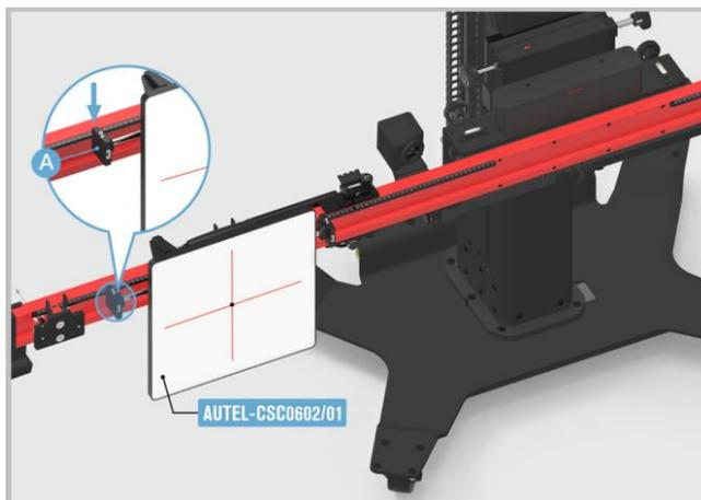
**Figure 6-14 Adjust the Reflector 2**
