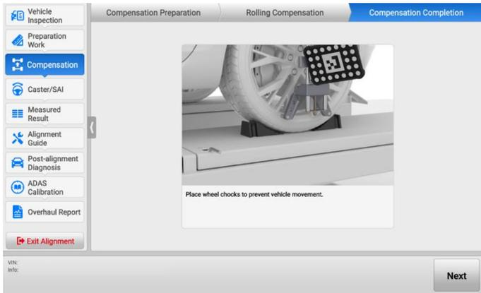
**Figure 4-40 Complete Rolling Compensation (Use Rim Clamp)**
