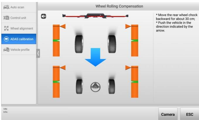
**Figure 6-93 Wheel Rolling Compensation 1**
