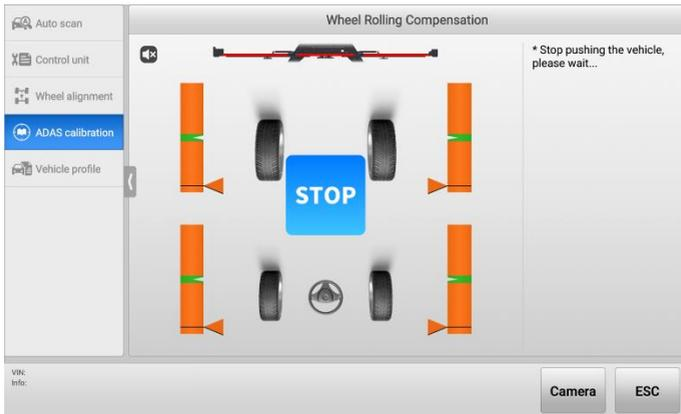
**Figure 6-95 Wheel Rolling Compensation 3**
