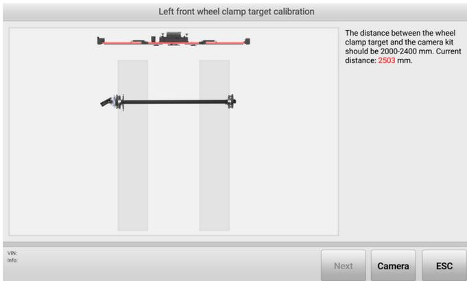
**Figure 5-22 Start Calibration (Use Calibration Bar) 1**
