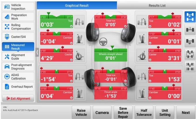
**Figure 5-66 Measured Result (Full Tolerance) Screen**
