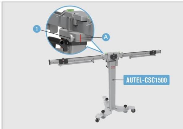
**Figure 3-21 Rotate the Fine Tuning Bolt**
